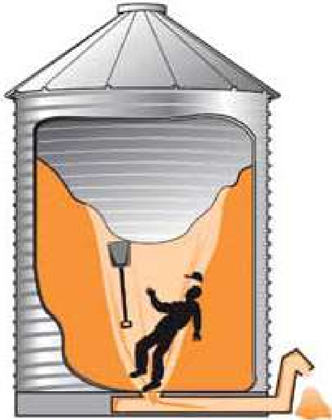
A center grain unloading auger draws grain from the top center and the grain forms a cone as the bin is emptied. Illustration: John A. Kramer, Safety Measures in Handling Stored Grain, Kansas State University, February 1989. Illustration: John A. Kramer, Safety Measures in Handling Stored Grain, Kansas State University.
